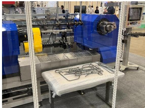
Rebar 3D processing machine
