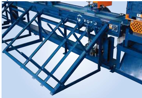
Storage rack standby arm is to receive finished products temporarily. After bundling, they can be discharged to the products storage rack.
