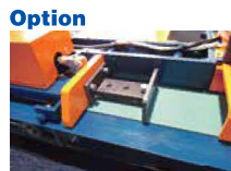
Option Shorter dimension can be cut with stopper for the short length
